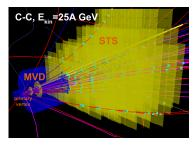
UrQMD central C-C, 25 A GeV ~ 24 tracks reconstructed with Cellular Automation and Kalman Filter algorithms
